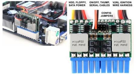
M3-ATX is an intelligent vehicle ATX power supply. Designed to provide power and to control the ON/OFF switch of a motherboard based on ignition status, M3-ATX is a wide input (6-24V) ATX power supply capable of surviving tough engine cranks (down to 5.7V) as well as transient over-voltage situations.
